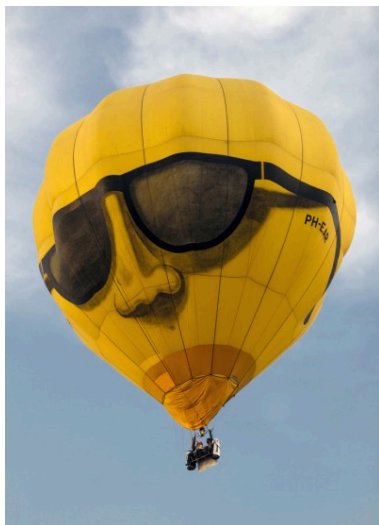
Figure 1. The air inside this hot air balloon flying over Putrajaya, Malaysia, is hotter than the ambient air. As a result, the balloon experiences a buoyant force pushing it upward. (credit: Kevin Poh, Flickr)
