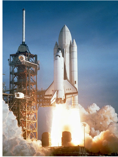
Figure 2. The space shuttle had a number of reusable parts. Solid fuel boosters on either side were recovered and refueled after each flight, and the entire orbiter returned to Earth for use in subsequent flights. The large liquid fuel tank was expended. The space shuttle was a complex assemblage of technologies, employing both solid and liquid fuel and pioneering ceramic tiles as reentry heat shields. As a result, it permitted multiple launches as opposed to single-use rockets. (credit: NASA)
