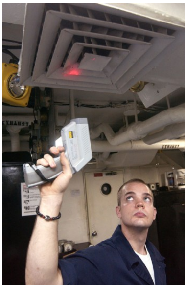
Figure 3. Fireman Jason Ormand uses a pyrometer to check the temperature of an aircraft carrier's ventilation system. (credit: Lamel J. Hinton/U.S. Navy)
