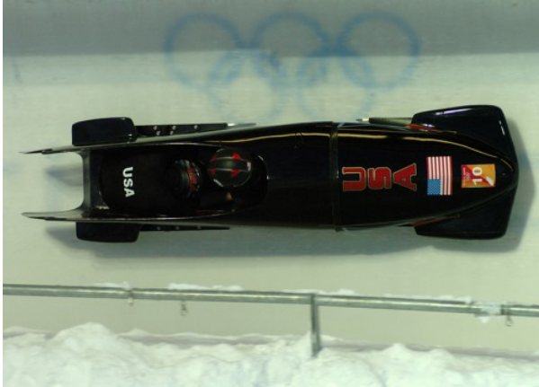
Figure 1. From racing cars to bobsled racers, aerodynamic shaping is crucial to achieving top speeds. Bobsleds are designed for speed. They are shaped like a bullet with tapered fins. (credit: U.S. Army, via Wikimedia Commons)
