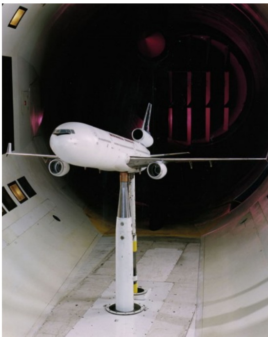
Figure 2. NASA researchers test a model plane in a wind tunnel. (credit: NASA/Ames)
