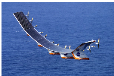
Figure 1. Solar energy is converted into electrical energy by solar cells, which is used to run a motor in this solar-power aircraft. (credit: NASA)
