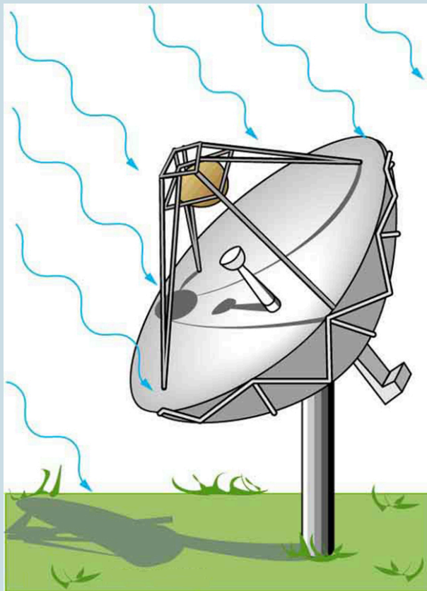
Figure 2. Satellite dishes receive TV signals sent from orbit. Although the signals are quite weak, the receiver can detect them by being tuned to resonate at their frequency.
