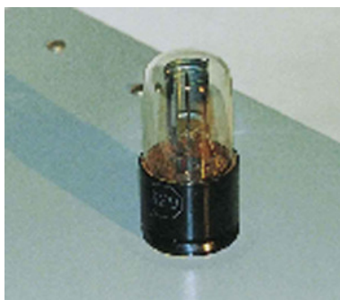
Figure 1. The photoelectric effect can be observed by allowing light to fall on the metal plate in this evacuated tube. Electrons ejected by the light are collected on the collector wire and measured as a current. A retarding voltage between the collector wire and plate can then be adjusted so as to determine the energy of the ejected electrons. For example, if it is sufficiently negative, no electrons will reach the wire. (credit: P.P. Urone)
