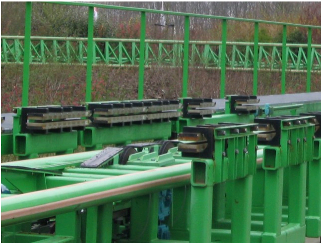
Figure 7. The rows of rare earth magnets (protruding horizontally) are used for magnetic braking in roller coasters. (credit: Stefan Scheer, Wikimedia Commons)
