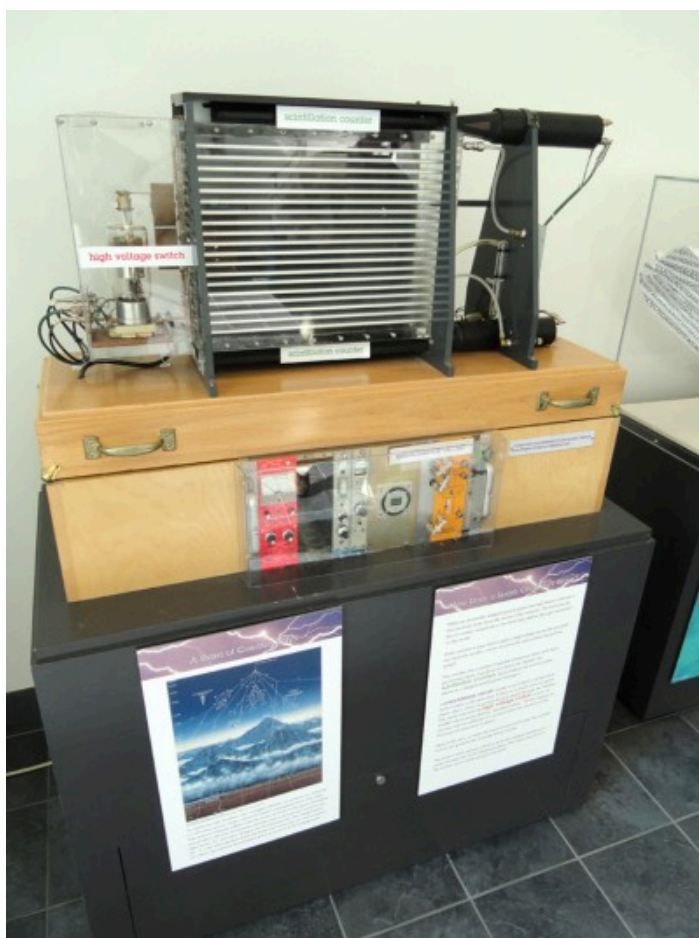
Figure 2. A spark chamber is used to trace the paths of high-energy particles. Ionization created by the particles as they pass through the gas between the plates allows a spark to jump. The sparks are perpendicular to the plates, following electric field lines between them. The potential difference between adjacent plates is not high enough to cause sparks without the ionization produced by particles from accelerator experiments (or cosmic rays). (credit: Daderot, Wikimedia Commons)
