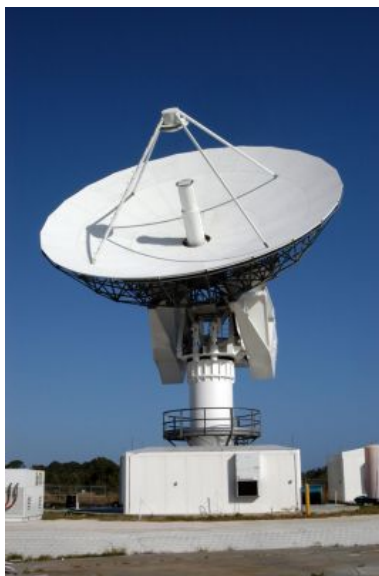
Figure 2. The electromagnetic waves sent and received by this 50-foot radar dish antenna at Kennedy Space Center in Florida are not visible, but help track expendable launch vehicles with high-definition imagery. The first use of this C-band radar dish was for the launch of the Atlas V rocket sending the New Horizons probe toward Pluto. (credit: NASA)
