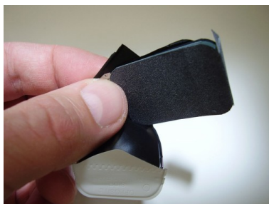
Figure 1. Film badges contain film similar to that used in this dental x-ray film and is sandwiched between various absorbers to determine the penetrating ability of the radiation as well as the amount. (credit: Werneuchen, Wikimedia Commons)
