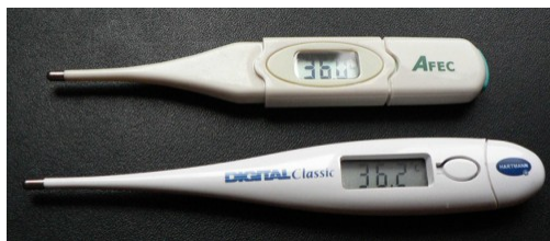
Figure 3. These familiar thermometers are based on the automated measurement of a thermistor's temperature-dependent resistance. (credit: Biol, Wikimedia Commons)
