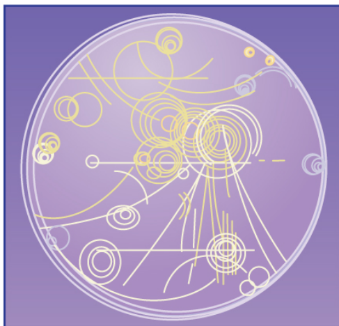
Figure 1. Trails of bubbles are produced by high-energy charged particles moving through the superheated liquid hydrogen in this artist's rendition of a bubble chamber. There is a strong magnetic field perpendicular to the page that causes the curved paths of the particles. The radius of the path can be used to find the mass, charge, and energy of the particle.
