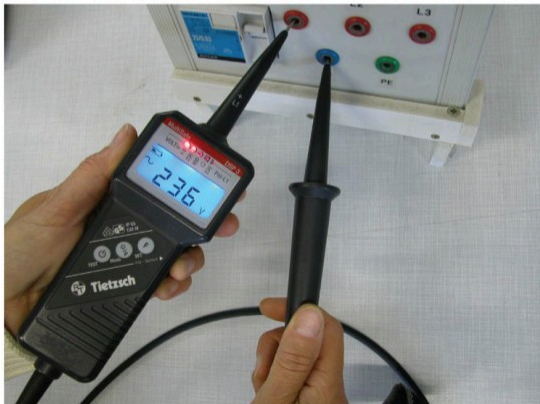
Figure 2. (a) To measure potential differences in this series circuit, the voltmeter (V) is placed in parallel with the voltage source or either of the resistors. Note that terminal voltage is measured between points a and b . It is not possible to connect the voltmeter directly across the emf without including its internal resistance, r . (b) A digital voltmeter in use. (credit: Messtechniker, Wikimedia Commons)
