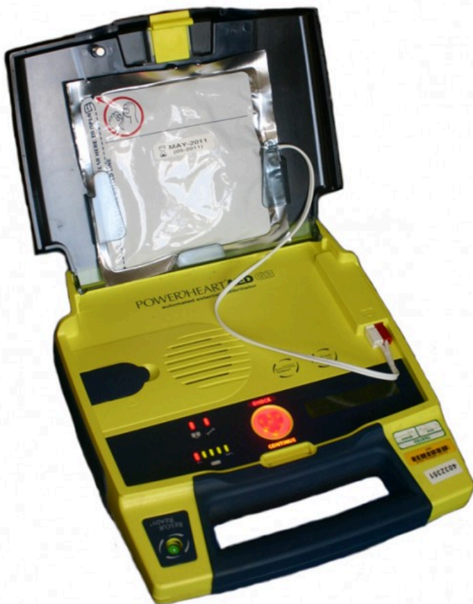
Figure 2. Automated external defibrillators are found in many public places. These portable units provide verbal instructions for use in the important first few minutes for a person suffering a cardiac attack. (credit: Owain Davies, Wikimedia Commons)
