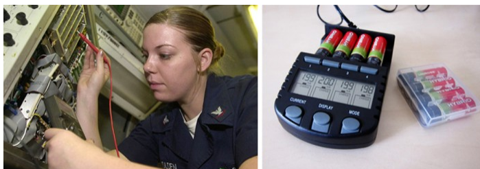
Figure 6. These two battery testers measure terminal voltage under a load to determine the condition of a battery. The large device is being used by a U.S. Navy electronics technician to test large batteries aboard the aircraft carrier USS Nimitz and has a small resistance that can dissipate large amounts of power. (credit: U.S. Navy photo by Photographer's Mate Airman Jason A. Johnston) The small device is used on small batteries and has a digital display to indicate the acceptability of their terminal voltage. (credit: Keith Williamson)
