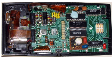
Figure 1. Energy stored in the large capacitor is used to preserve the memory of an electronic calculator when its batteries are charged. (credit: Kucharek, Wikimedia Commons)
