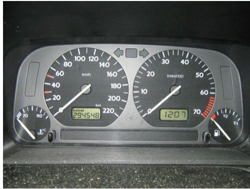
Figure 1. The fuel and temperature gauges (far right and far left, respectively) in this 1996 Volkswagen are voltmeters that register the voltage output of “sender” units, which are hopefully proportional to the amount of gasoline in the tank and the engine temperature. (credit: Christian Giersing)
