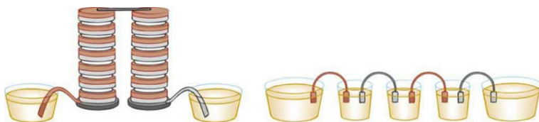
Figure 9. Batteries are multiple connections of individual cells, as shown in this modern rendition of an old print. Single cells, such as AA or C cells, are commonly called batteries, although this is technically incorrect.
