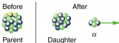
Figure 2. Alpha decay is the separation of a {}^4\text{He} nucleus from the parent. The daughter nucleus has two fewer protons and two fewer neutrons than the parent. Alpha decay occurs spontaneously only if the daughter and {}^4\text{He} nucleus have less total mass than the parent.
