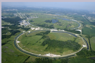
Figure 4. The Fermi National Accelerator Laboratory, near Batavia, Illinois, was a subatomic particle collider that accelerated protons and antiprotons to attain energies up to 1 Tev (a trillion electronvolts). The circular ponds near the rings were built to dissipate waste heat. This accelerator was shut down in September 2011. (credit: Fermilab, Reidar Hahn)
