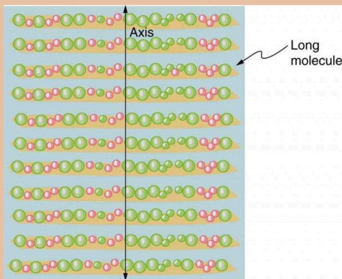
Figure 9. Long molecules are aligned perpendicular to the axis of a polarizing filter. The component of the electric field in an EM wave perpendicular to these molecules passes through the filter, while the component parallel to the molecules is absorbed.
