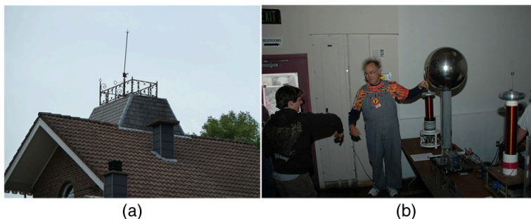
Figure 8. (a) A lightning rod is pointed to facilitate the transfer of charge. (credit: Romaine, Wikimedia Commons) (b) This Van de Graaff generator has a smooth surface with a large radius of curvature to prevent the transfer of charge and allow a large voltage to be generated. The mutual repulsion of like charges is evident in the person's hair while touching the metal sphere. (credit: Jon 'ShakataGaNai' Davis/Wikimedia Commons).
