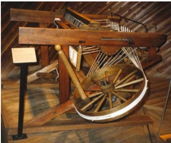
Model of spinning jenny in the Museum of Early Industrialization, Wuppertal
