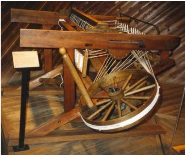
Model of the spinning jenny in a museum in Wuppertal. Invented by James Hargreaves in 1764, the spinning jenny was one of the innovations that started the revolution.
