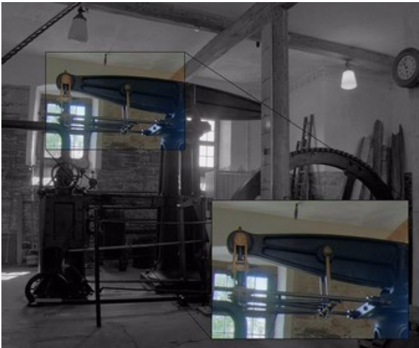
Watt's parallel motion on a pumping engine
