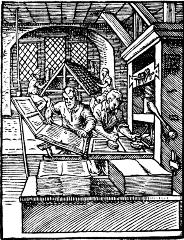
Early wooden printing press, depicted in 1568: Such presses could produce up to 240 impressions per hour. At the left in the foreground, a “puller” removes a printed sheet from the press. The “beater” to his right is inking the form. In the background, compositors are setting type.
