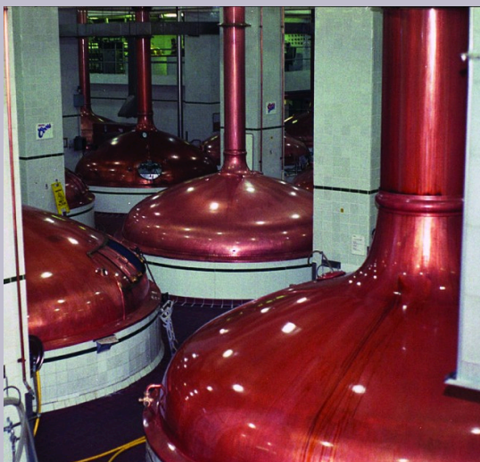
Figure 3. An oxide of carbon is removed from these fermentation tanks through the large copper pipes at the top. (credit: "Dual Freq"/Wikimedia)
