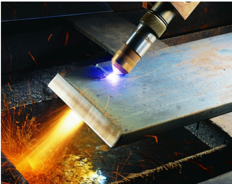
Figure 2. A plasma torch can be used to cut metal. (credit: “Hypertherm”/Wikimedia Commons)
