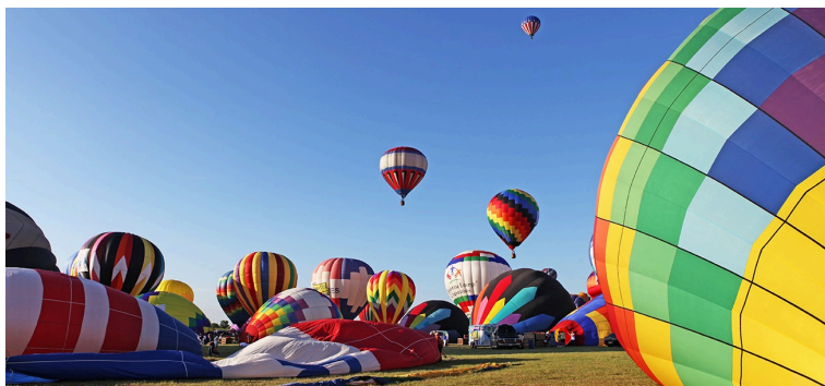
Figure 1. The hot air inside these balloons is less dense than the surrounding cool air. This results in a buoyant force that causes the balloons to rise when their guy lines are untied. (credit: modification of work by Anthony Quintano)
