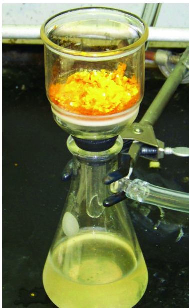
Figure 2. Precipitate may be removed from a reaction mixture by filtration.
