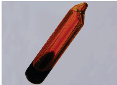
Figure 4. An equilibrium is pictured between liquid bromine, \text{Br}_2(l) , the dark liquid, and bromine vapor, \text{Br}_2(g) , the orange gas. Because the container is sealed, bromine vapor cannot escape and equilibrium is maintained. (credit: http://images-of-elements.com/bromine.php )
