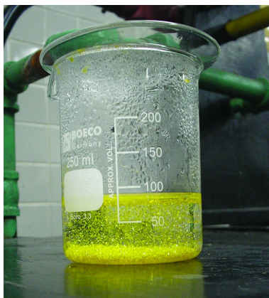
Figure 1. A precipitate of \text{PbI}_2 forms when solutions containing \text{Pb}^{2+} and \text{I}^- are mixed. (credit: Der Kreole/Wikimedia Commons)
