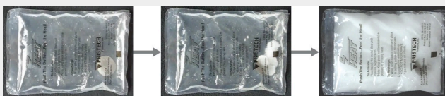
Figure 5. Chemical hand warmers produce heat that warms your hand on a cold day. In this one, you can see the metal disc that initiates the exothermic precipitation reaction. (credit: modification of work by Science Buddies TV/YouTube)
